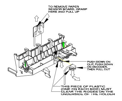
Figure 5-8. Paper and Encoder Sensor Removal.
